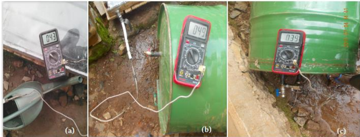
Figure 4. Performance evaluation of the final manufactured TSWH system. Temperature evaluation of the sensor (a), temperature evaluation of the TSWH system at the exit point of the sensor (b) and temperature evaluation of the TSWH system at the exit point of the storage tank (c).
